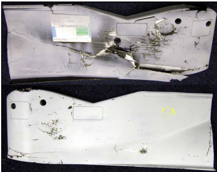
Figure 3: Despite suffering the same fate as the specimen in Figure 2, the Innegra/Carbon front wing endplate remained intact and relatively unscathed.
